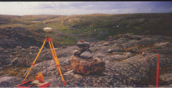
(Left) A GPS station was set up on a parcel corner monument. This station received signals from orbiting satellites which allowed the Ontario Land Surveyor to accurately compute the precise location of the corner.
