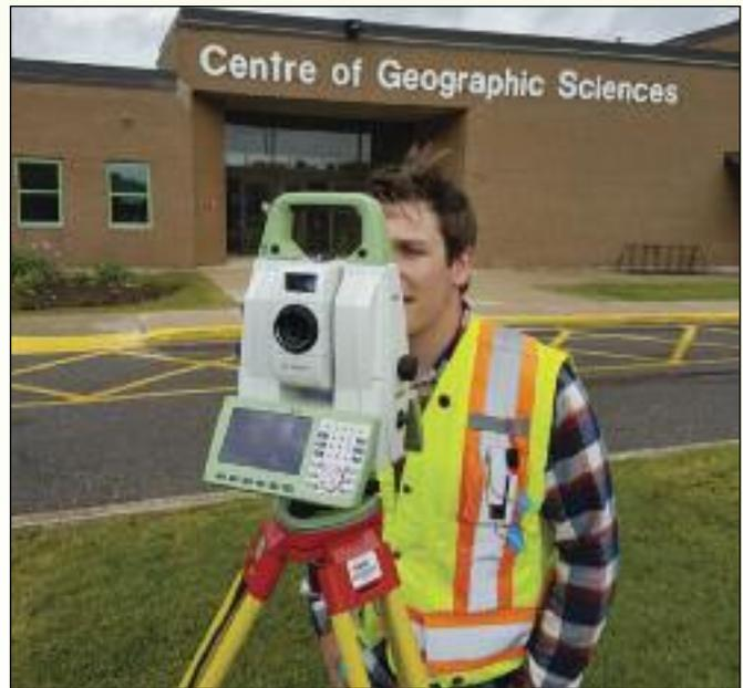
Dylan MacDonald using the Leica Nova MS60 Multistation – Scanner/Robotic Total Station
