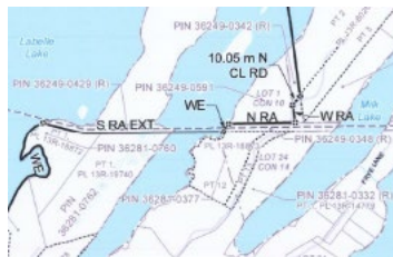
Caption: Example of a descriptive plan for Frontenac Provincial Park demonstrating the complex and precise location of the regulated area extents. The boundary from left to right, follows the Water’s Edge (WE) to the Southern limit of the road allowance and extended (S RA EXT) to the intersection of the Water’s Edge (WE), to the Northern limit of the road allowance 8 (N RA), to the western limit of the road allowance (W RA), to 10.05 m North of the centreline of the road (10.05 m N CL RD). Descriptive plans support the legal description for regulated boundaries, including provincial parks, conservation reserves, wildlife management units, fish management zones and much more.
